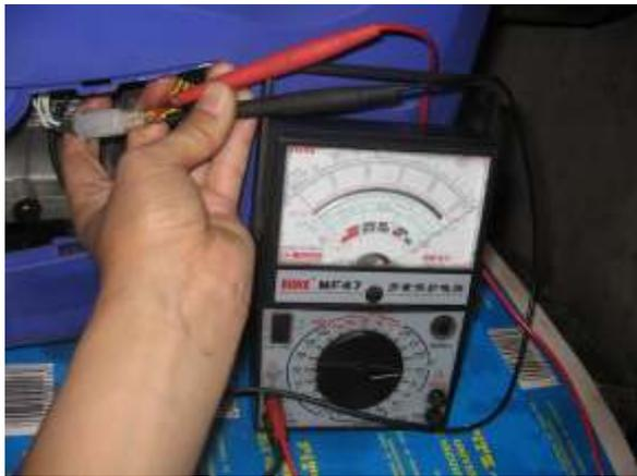
Picture 2. The ignition coil when the generator shut down no electric, then pull the starter (the normal AC voltage about 10V.)
