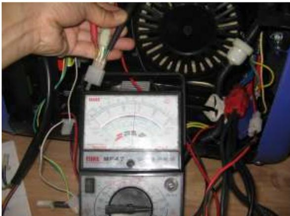
Picture 3. Trigger coil Green, Yellow/green wires do not circulate.
