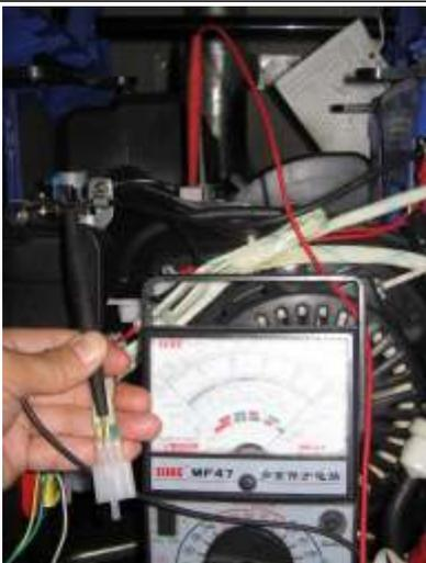
Picture 4. No resistance value (The normal is about 50 ohm) , if the white wire and engine crust do not circulate, it will result in non-ignition.
