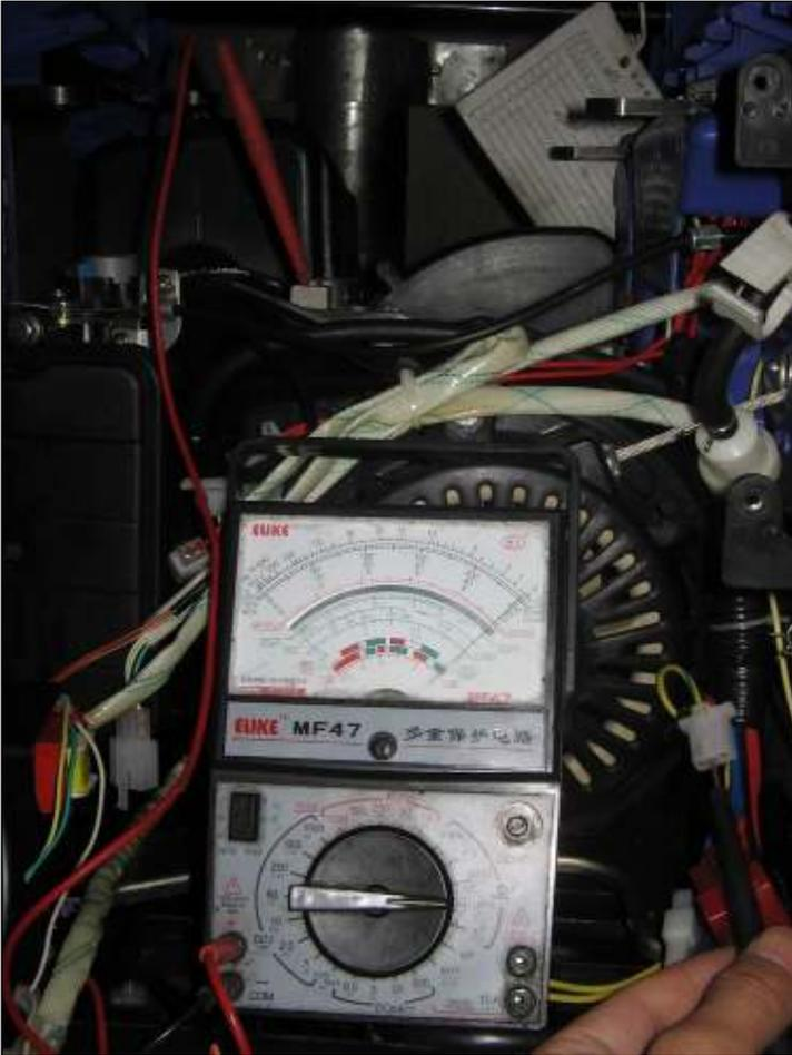
Picture 4. Yellow/Green wire and engine crust do not circulate.
