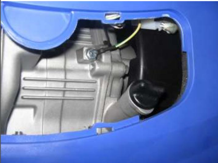
Picture 5. The ground wire not connecting or damage.
